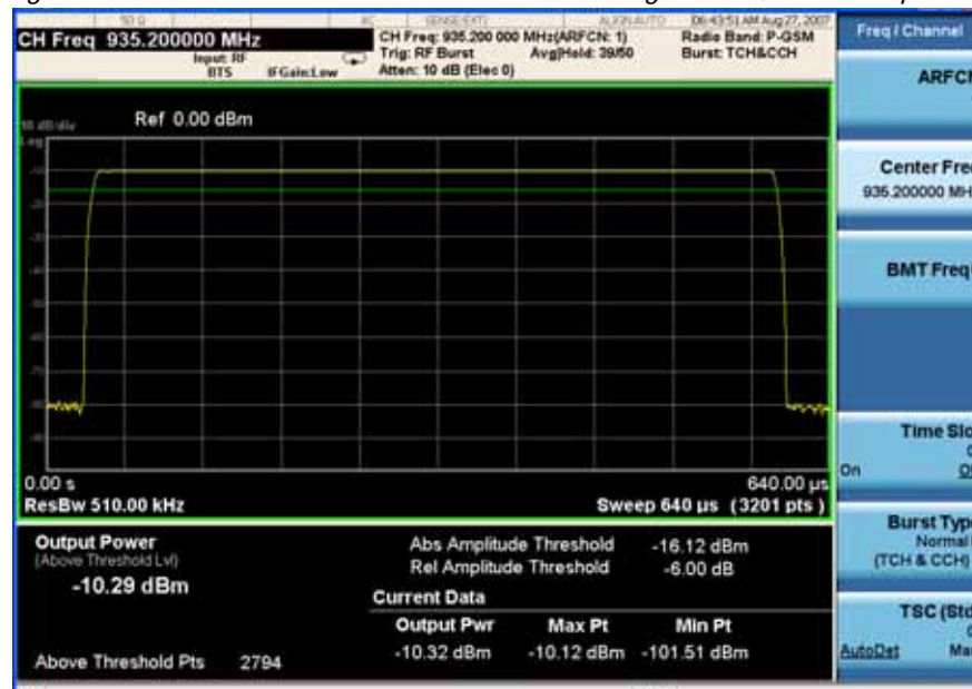
Figure 2-2 Transmit Power Result - Single Burst, RF Envelope
